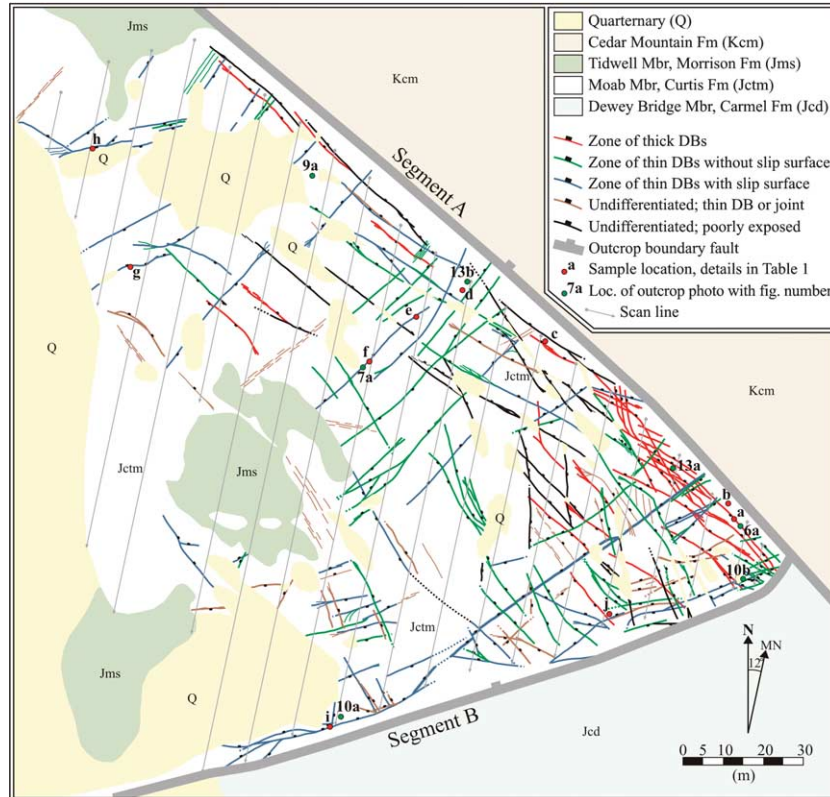
Fig. 4. Structural outline of the Courthouse Branch Point locality. Only the most laterally continuous structures are shown at this scale. Deformation bands (DBs) and slip surfaces dominate the damage zone. The presence of joints has been indicated, but not verified at the scale of mapping shown here. Thick lineaments represent zones of sub-parallel deformation structures, whereas thin lineaments represent single structures.
